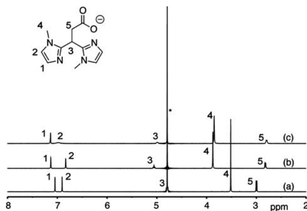
Fig. 3 400 MHz 1 H NMR spectra of the titration of K[MIm 2 Pr] with ZnCl 2 in D 2 O at room temperature: a K[MIm 2 Pr]; b K[MIm 2 Pr] and ZnCl 2 2:1; c K[MIm 2 Pr] and ZnCl 2 1:1. Asterisks denote the residual solvent peak
