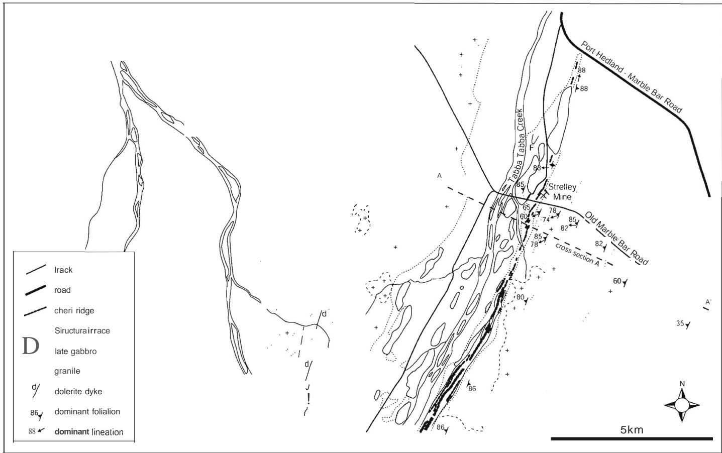
Aerial photograph interpretation, with added field structural and kinematic data. Location indicated in Figure 7.5. Full version on CD.
