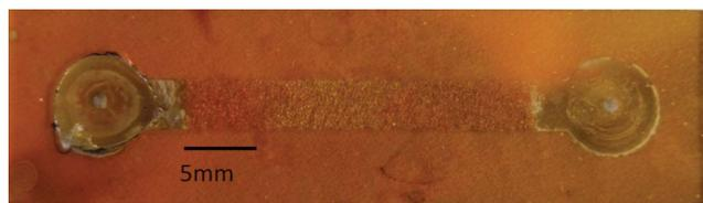
**Fig. 2** Picture of a micro-model with 3000 pore bodies and 9000 pore throats with a mean pore size of 70  $\mu\text{m}$ . The two round reservoirs and the holes for introduction and removal of the two fluids are visible too.
