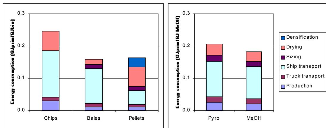
**Figure 5.9: Chain energy consumption figures for a Latin-American situation with a coastal CGP in  $GJ_{prim}/GJ_{bio}$  (woody biomass) or  $GJ/GJ_{fuel}$  (liquid fuels); international transport distance 10,000 km; ship transport only.**
