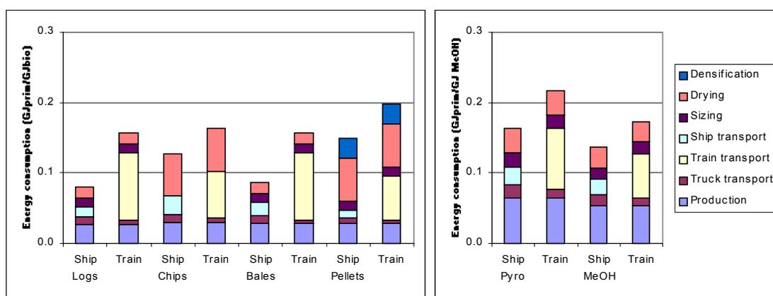
**Figure 5.4: Chain energy consumption figures for a European situation with a coastal CGP in  $GJ_{\text{prim}}/GJ_{\text{bio}}$  (woody biomass) or  $GJ/GJ_{\text{fuel}}$  (liquid fuels); international transport distance 1500 km.**
