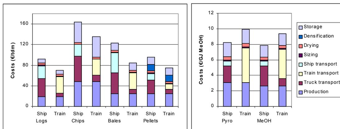
**Figure 5.1: Chain costs for a European situation with an inland CGP in €/t<sub>dm</sub> (woody biomass) or €/GJ<sub>fuel</sub> (liquid fuels); international transport distance 1500 km; conversion costs are excluded.**
