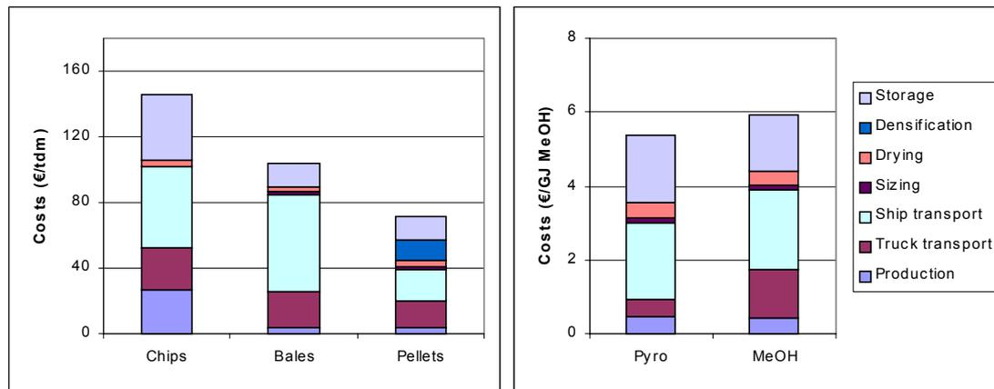
**Figure 5.7: Chain costs for a Latin-American situation with a coastal CGP in €/t<sub>dm</sub> (woody biomass) or €/GJ<sub>fuel</sub> (liquid fuels); international transport distance 10,000 km; conversion costs are excluded; ship transport only.**
