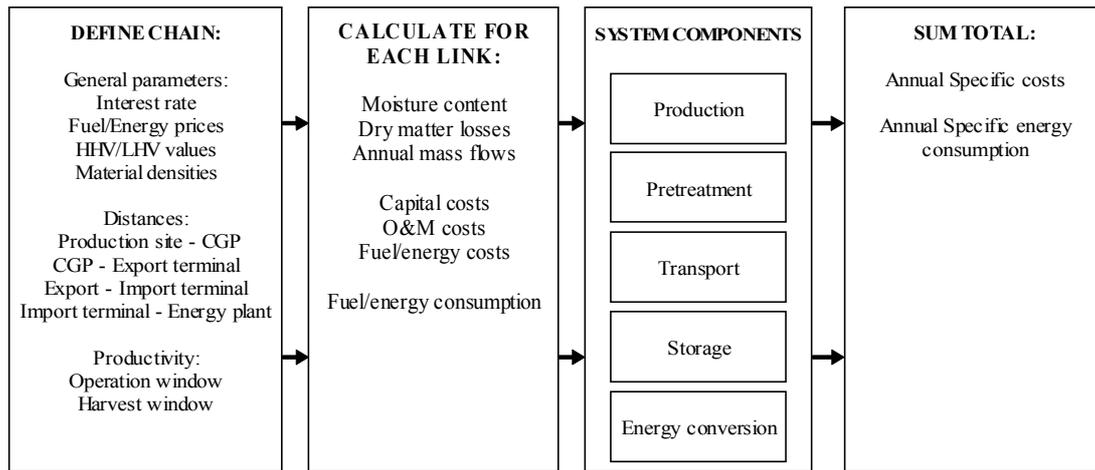
**Figure 2.3: Schematic representation of the model.**
