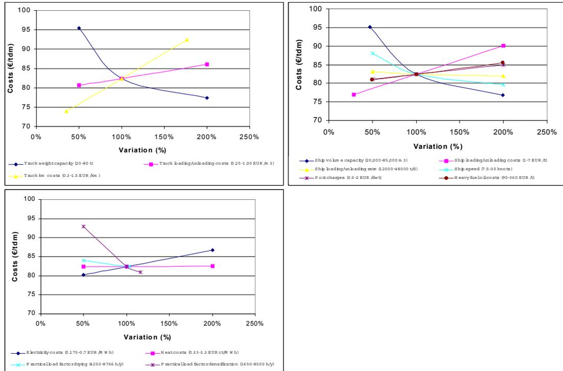
**Figure 5.14: Sensitivity analysis for uncertain input data concerning truck transport, ship transport and pretreatment operations; the default position is the pellets chain for Latin-America and an inland CGP.**
