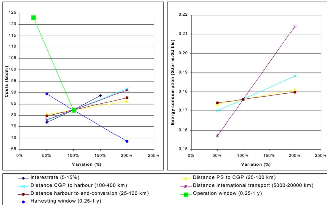
**Figure 5.12: Sensitivity analysis with regard to interest rate, scale, distance production site; the default position is the pellets chain for Latin-America and an inland CGP.**
