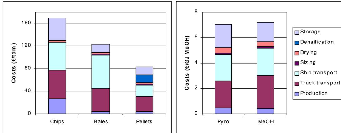
**Figure 5.6: Chain costs for a Latin-American situation with an inland CGP in €/t<sub>dm</sub> (woody biomass) or €/GJ<sub>fuel</sub> (liquid fuels); international transport distance 10,000 km; conversion costs are excluded; ship transport only.**
