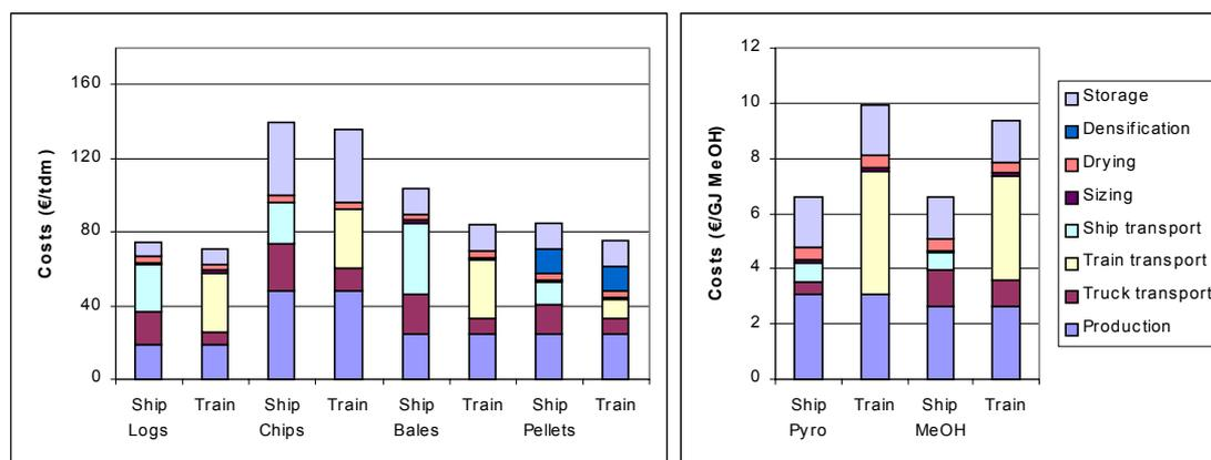
**Figure 5.2: Chain costs for a European situation with a coastal CGP in €/t<sub>dm</sub> (woody biomass) or €/GJ<sub>fuel</sub> (liquid fuels); international transport distance 1500 km; conversion costs are excluded.**
