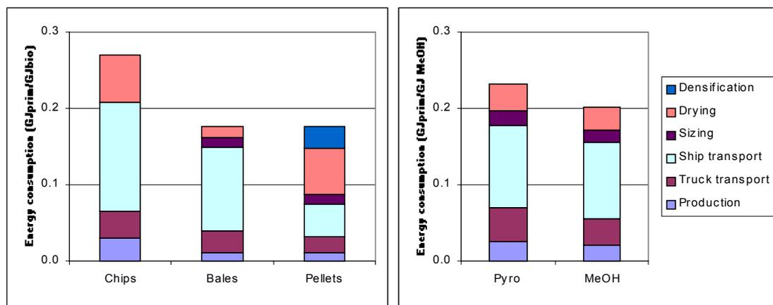
**Figure 5.8: Chain energy consumption figures for a Latin-American situation with an inland CGP in  $GJ_{prim}/GJ_{bio}$  (woody biomass) or  $GJ/GJ_{fuel}$  (liquid fuels); international transport distance 10,000 km; ship transport only.**
