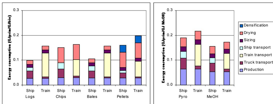
**Figure 5.3: Chain energy consumption figures for a European situation with an inland CGP in  $GJ_{\text{prim}}/GJ_{\text{bio}}$  (woody biomass) or  $GJ/GJ_{\text{fuel}}$  (liquid fuels); international transport distance 1500 km.**
