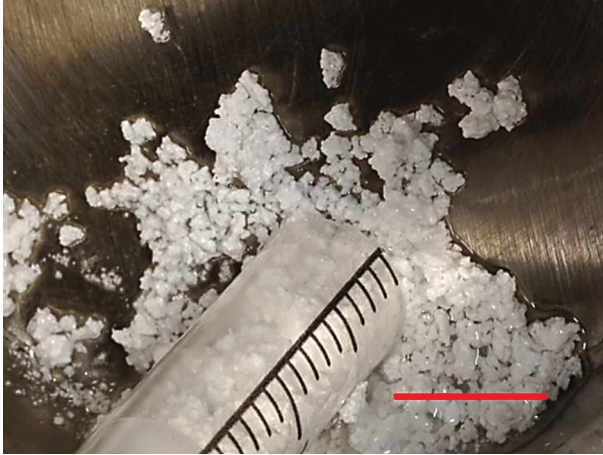
FIGURE 1: 1-2 mm sized micro structured calcium phosphate particles. (red scale bar: 1 cm)
