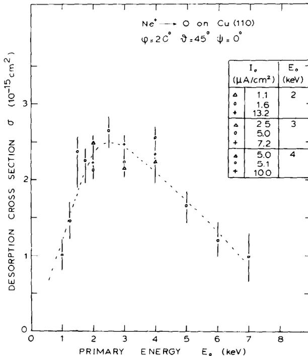
Fig. 4. Cross sections for the desorption of adsorbed O on Cu(110) by Ne<sup>+</sup> ion bombardment as a function of the primary ion energy (ion scattering method).
