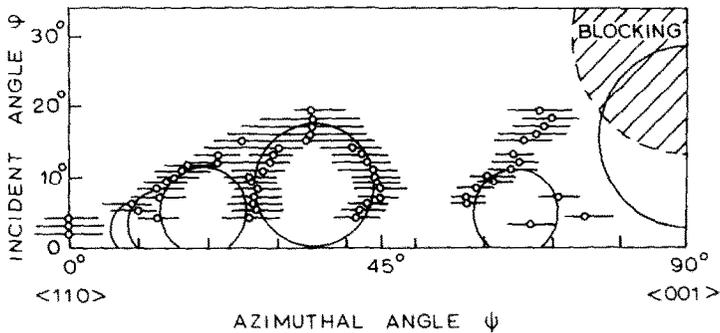
Fig. 2. A  $\varphi$ - $\psi$  diagram of the peak positions as deduced from curves shown in fig. 1. (○) peak position with bar indicating the peak width. The circles represent the shadow cones calculated for different copper lattice atoms in the neighbourhood of an adsorbed O atom situated 0.6 Å below the midpoint between two adjacent Cu atoms in an (001) surface row.
