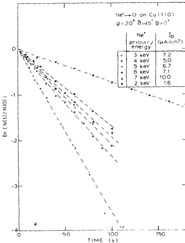
Fig. 3. Decrease of the normalized scattering yield from an oxygen exposed (1000 L) Cu(110) surface due to Ne<sup>+</sup> ion bombardment, plotted as a function of the bombarding time.
