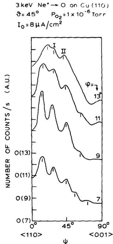
Fig. 1 Measured yields of  $\text{Ne}^+$  ions scattered by O atoms chemisorbed on a Cu(110) surface as a function of the azimuthal angle  $\psi$  for the various angles of incidence  $\phi$  indicated. The curves are separated by a vertical shift of the origin  $O(7)$ ,  $O(9)$ , ...).
