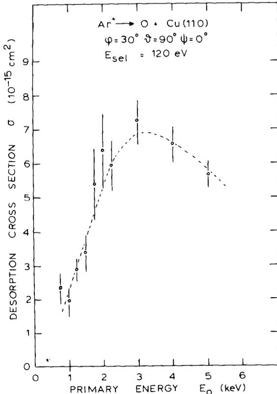
Fig. 5. Cross sections for the desorption of adsorbed O on Cu(110) by  $\text{Ar}^+$  ion bombardment as a function of the primary ion energy (secondary ion method).
