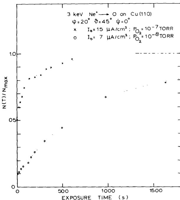
Fig. 6. Normalized number of counts for  $\text{Ne}^+$  ions scattered by O as a function of the time that the copper surface is exposed to oxygen with the ion beam off, measured directly after the onset of the  $\text{Ne}^+$  ion beam.
