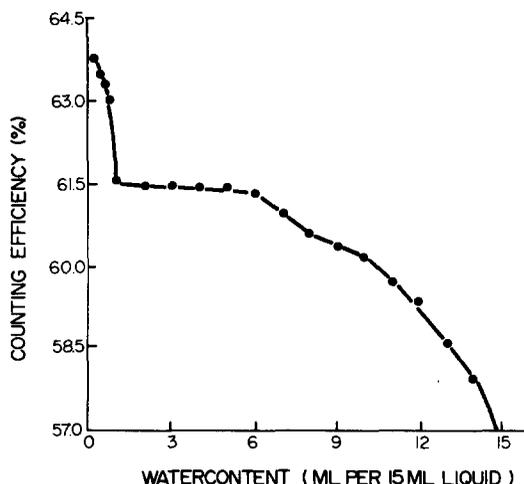
FIG. 8. Detection efficiency of  $^{32}\text{P}$ -Čerenkov radiation in ethanol and the effect of increasing amounts of water.
