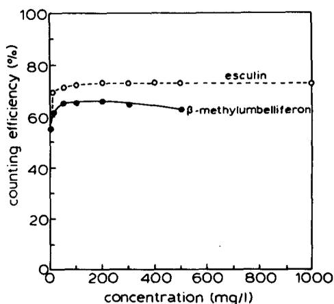
FIG. 2. Counting efficiency as a function of the concentration of wavelength shifters esculin and  $\beta$ -methyl umbelliferon. Polyethylene vials, content 10 ml;  $\text{Na}_2\text{H}^{32}\text{PO}_4$  in distilled water at pH 7.0; amplifier gain 30%.
