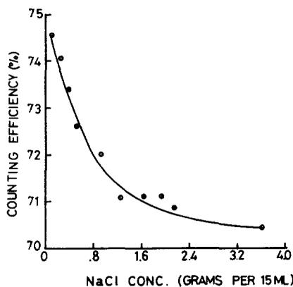
FIG. 4. The effect of salt on the function of the wavelength shifter sodium salicylate. Sodium salicylate concentration 200 g/l. Other counting conditions as described in the caption to Fig. 2.
