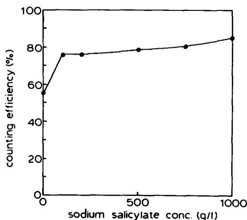
FIG. 3. Counting efficiency as a function of the concentration of the wavelength shifter sodium salicylate. Counting conditions as described in the caption to Fig. 2.
