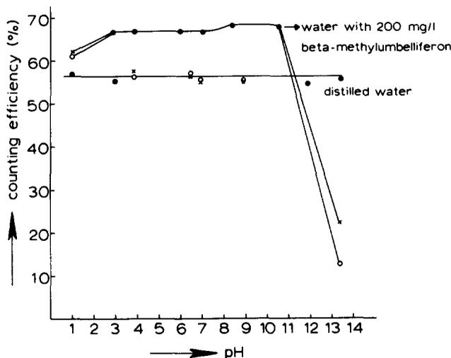
FIG. 5. The effect of pH on the function of  $\beta$ -methyl umbelliferon as wavelength shifter. (x) measured immediately after preparation of the samples; (O) measured upon two weeks storage of the samples. 200 mg/l  $\beta$ -methyl umbelliferon; other counting conditions as described in the caption to Fig. 2. For comparison the same measurements in distilled water only are given in this figure as well.
