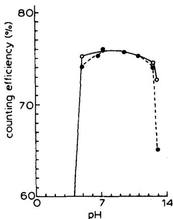
FIG. 7. The effect of pH on the function of the wavelength shifter sodium salicylate. (O) measured immediately after preparation of the samples; (●) measured upon two weeks storage of the samples. 200 g/l sodium salicylate; other counting conditions as described in the caption to Fig. 2.
