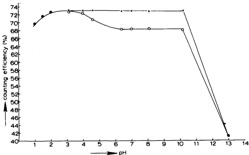
FIG. 6. The effect of pH on the function of the wavelength shifter esculin. (x) measured immediately after preparation of the samples; (O) measured upon two weeks storage of the samples. 400 mg esculin/l; counting conditions as described in the caption to Fig. 2.
