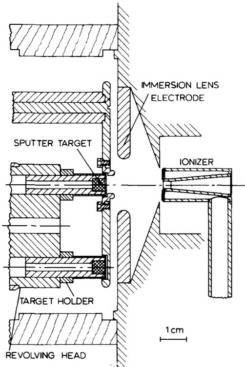
Fig. 4. The modified inverted sputter source.
