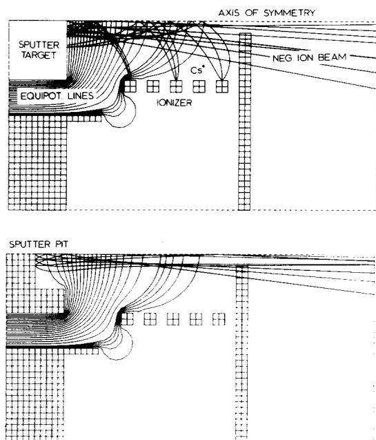
Fig. 2. (a) Plotted equipotential lines and trajectories of the negative ions for a flat sputter target. (b) The same for a sputter target with a pit.
