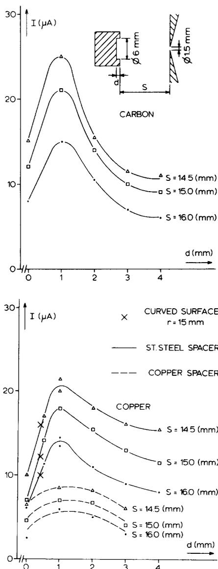
Fig. 3. (a) Variation of C<sup>-</sup> current as a function of the depth  $d$  of the pit with different spacings  $S$ . (b) The same for Cu<sup>-</sup>. Solid lines: high surface temperature, dotted lines: low surface temperature. Crosses: curved sputter surface (see text).
