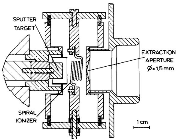
Fig. 1. The modified ion source. A spiral ionizer is used in an ANIS source geometry.
