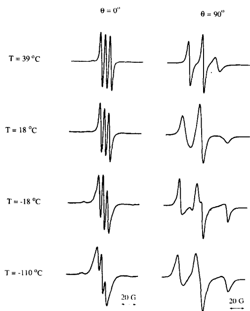
Fig. 3. EPR spectra of ^{14}\text{N} -CSL in DMPC/cholesterol (2:1) bilayers, recorded at various temperatures with \theta = 0^\circ ( \mathbf{H}_0 \parallel \mathbf{n} ) and \theta = 90^\circ ( \mathbf{H}_0 \perp \mathbf{n} ) respectively. Each temperature represents a motional regime: T = 39^\circ\text{C} : motional narrowing; T = 18^\circ\text{C} : slow motion; T = -18^\circ\text{C} : rigid limit; T = -110^\circ\text{C} : rigid limit with dominant broadening.
