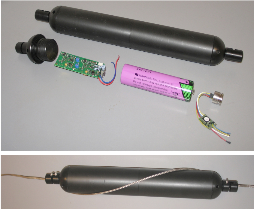
Figure 3. a) A probe and its internal components (the transmitter, lithium battery and a pressure sensor) and b) a probe attached to the 3 mm kevlar rope.
