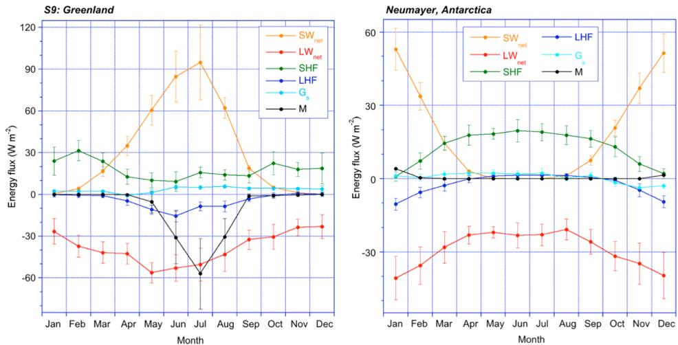
**Figure 1.** Seasonal cycle (based on monthly means) of SEB components at AWS S9 situated on the Greenland ice sheet (67°03' N, 48°14' W, 1520 m asl, data period 1 Sep. 2003 - 31 Jul. 2010) and Neumayer station in Antarctica (70°39' S, 8°15' W, 40 m asl, data period 1 Jan. 1995 - 31 Dec. 2007). Error bars indicate standard deviation of the monthly means. Note the difference in vertical scales.
