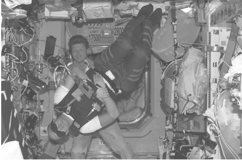
Figure 9.1. The test astronaut and the assisting crew member in the task in which the test astronaut is rotated like the hour hand of a clock. The vest worn by the astronaut included 56 small vibrators. The location of vibration indicated the direction of down. Here, the vibrator on his right shoulder is active. (Photo NASA/ESA).
