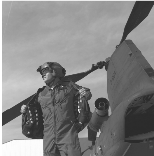
Figure 1.1. A helicopter pilot showing a TNO Tactile Torso Display (TTTD) to support local guidance. The TTTD consists of a matrix of vibrating elements inside a multi-ply garment covering the pilot's torso. By using the skin as an information channel, this navigation display can potentially reduce the overload of the pilot's ears and eyes. Furthermore, the localized vibrations can act as a 'tap-on-the-shoulder' and may be intuitively processed by the pilot, thus reducing the risk of cognitive overload.
