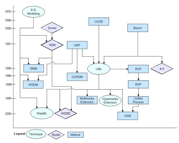
Figure 3-2: Relations between design methods, models and techniques
