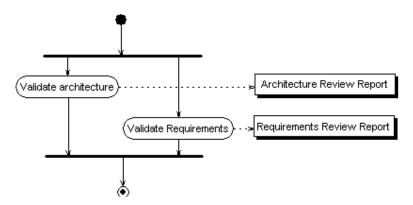
Figure 11-7: Meta-model validation workflow
