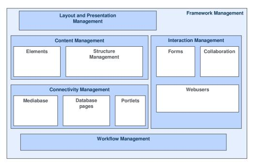
Figure 5-1: GX WebManager architecture
