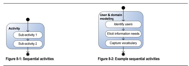
In Figure 8-2 an example from practice is illustrated. The example is taken from the requirements capturing workflow in UML-based Web Engineering. The main activity, user & domain modeling, consists of three activities that need to be carried out in a predefined order
