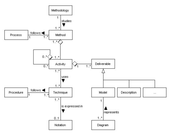
Figure 4-1: Meta-model of method engineering concepts
