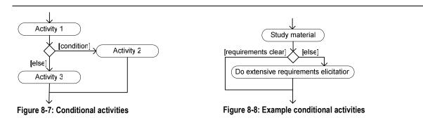
In Figure 8-8 an example from practice is illustrated. A requirements analysis at GX starts with studying the material. Based on this study, the decision is taken whether to do an extensive requirements elicitation session or not. The condition for not carrying out this requirements session is represented at the left of the branch, namely [requirements clear]. If this condition is not met, [else], the other arrow is followed.
