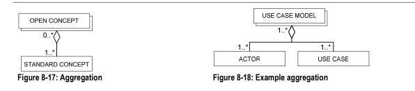
In Figure 8-18 aggregation is exemplified by a fragment of the requirements capture workflow in UML-Based Web Engineering. A USE CASE MODEL consists of one or more ACTORS and USE CASES.
