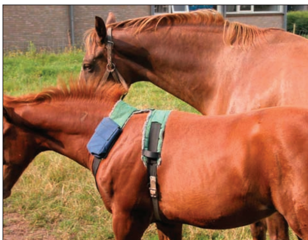
Figure 1—Photograph of a 3-month-old foal with a harness used to carry GPS equipment.
