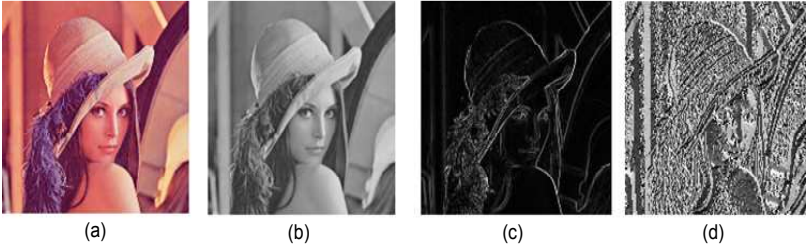
Figure 2.3: The original image (a) is converted to gray scale signal with \sigma = 1.0 (b) after that gradients, which are represented by its magnitude (c) and orientation (d) are computed.
