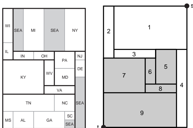
Figure 6: An L-shape destructible layout of the Eastern US. The shaded area shows the L-shaped polygon after the removal of rectangles 1 – 4.
