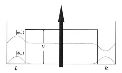
FIG. 1. A proton is in superposition  $|\phi_+\rangle$  of two states localized in boxes L and R. In between the boxes there is an external constant potential V which lifts the degeneracy of  $|\phi_+\rangle$  and  $|\phi_-\rangle$ . When the location of the proton is measured protectively, by sending an electron through the middle between the boxes, the electron will pass the boxes on a straight trajectory.
