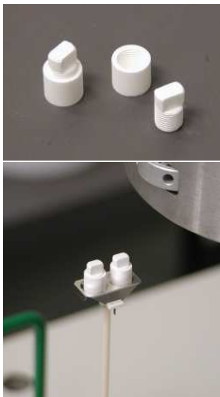
Figure 4.2: Boron crucibles as used in the DTA experiments. The height is 8 mm, the outer diameter is 6.5 mm.
