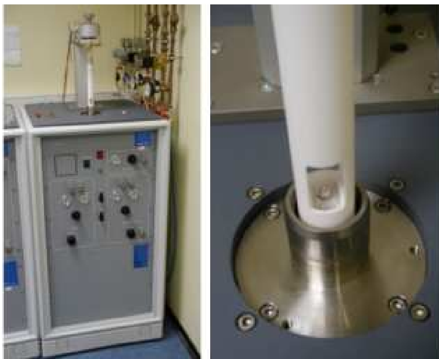
Figure 2.1: The Setaram Multi-HTC calorimeter, with a closeup from the detector.
