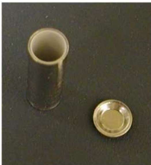
Figure 2.3: The platinum crucibles with a cover and a boron nitride liner, as used in the experiments.
