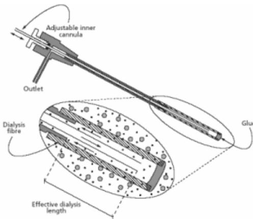
Fig. 2 Schematic drawing of a microdialysis probe
