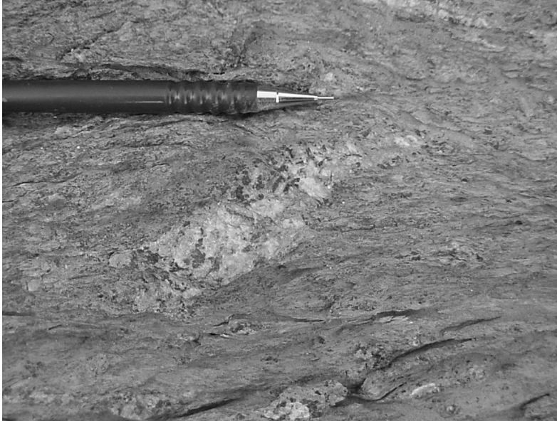
Figure 4-8 A rotated diorite clast indicates a dextral sense of shear.
