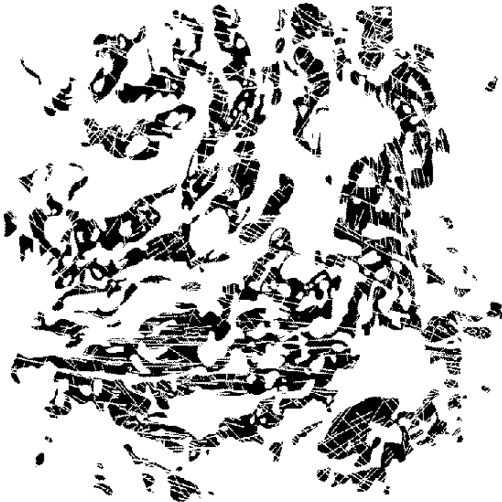
Figure 1.1: Fractures in 160 m. by 160 m. granitic rock of the Lac du Bonnet batholith in Manitoba. From Stone, Kaminen and Brown (1984). Digitized and post-processed by professor A.J. Baddeley of the University of Western Australia. The irregular black region is the rock's surface. The white parts represent areas where the rock cannot be observed due to soil, vegetation or water. The white lines through the black regions indicate fractures.
