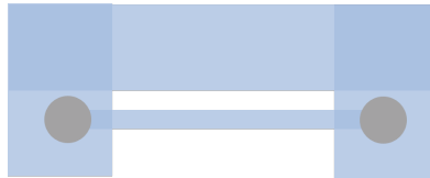
Figure 4.1: Schematic of sample for optimal arrest of the colloidal dispersion. The sample was prepared by gluing two ends of a microscope slide onto a half of a microscope slide cut over its long axis, onto which a capillary with the particle dispersion was glued using UV glue. The sample configuration enables the simultaneous imaging and exposure to UV light of the dispersion, without obstructing of the thick microscope slide glass.
