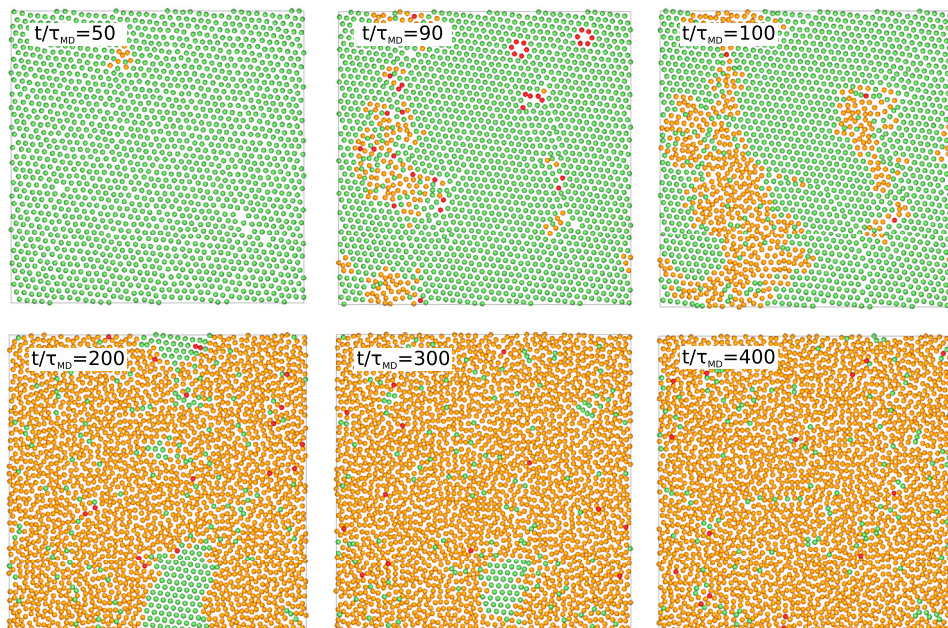
FIG. 13. Top view of the first layer of the sediment showing the melting of the hexagonal phase to a fluid for varying t/\tau_{MD} as labeled. The particles are coloured according to their individual BOO, namely, quasicrystal (red), square (purple), hexagon (green), and fluid (orange).
