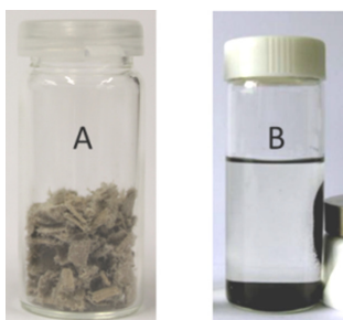
Figure 2.14: Holocellulosic fractions derived from two different Ni-catalysed up-stream processes: (A) RaneyNi catalysed removal of lignin from Poplar wood chips (pulp conducive to further downstream processing 198 ), and; (B) Ni/C catalysed removal of lignin from Birch wood saw dust (pulp not conducive to enzymatic hydrolysis 281 ). Image A reproduced with permission from Angew. Chem. Int. Ed. , 2014, 53 , 8634-8639. Copyright 2014 John Wiley and Sons. Image B reproduced with permission from Energ. Environ. Sci. , 2013, 6 , 994-1007. Copyright 2013 Royal Society of Chemistry.
