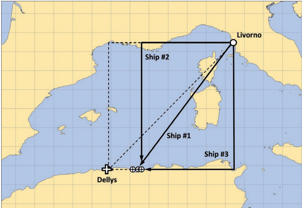
Figure 3.2 - Correct location of Dellys on a plane chart and the three locations where it would be charted as a result of plane charting.
