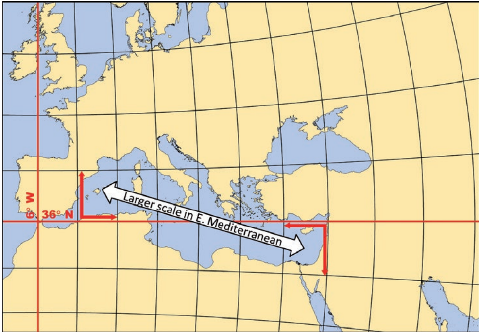
Figure 6.7 - Oblique stereographic projection of the Mediterranean area with projection centre at latitude 36^{\circ} S and longitude 6^{\circ} W.
