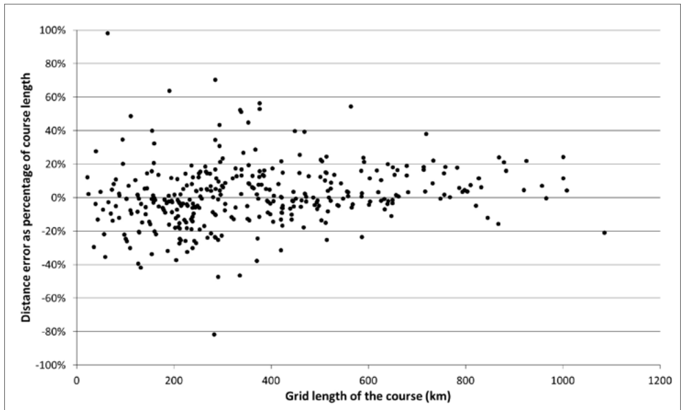
Figure 8.26 – Distance errors in the peleio when treated as scaled off.
