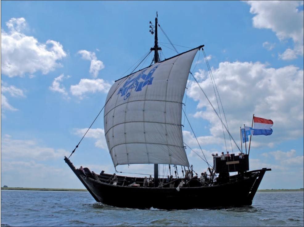
Figure 4.11 - Kampen Cog, sailing close-hauled; the three strips that constitute the lower half of the sail are detachable 'bonnets' (©Stichting Kamper Kogge; reproduced with permission).
