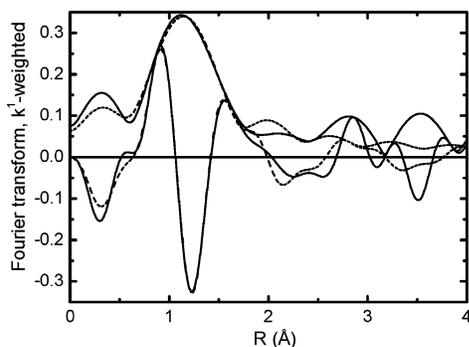
**Figure 2.** Absolute and imaginary parts of the Fourier transform and best fit (dashed line) obtained for dehydrated H-Y zeolite using one long and three short Al-O bonds. The Fourier transform is  $k^1$ -weighted, and the Fourier range is  $2.74 < k < 8$  Å<sup>-1</sup>; the fit is performed in  $R$ -space:  $0 < R < 1.8$  Å.
