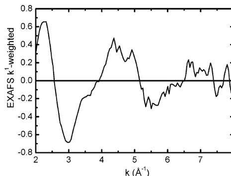
Figure 1.  $k^1$ -Weighted normalized Al K edge EXAFS data of NH<sub>4</sub>-Y zeolite.
