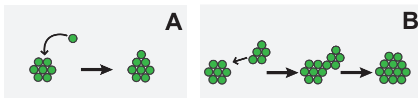
Figure 2.8. Growth mechanisms of NCs: (a) growth by monomer addition, (b) growth by coalescence of smaller NCs.
