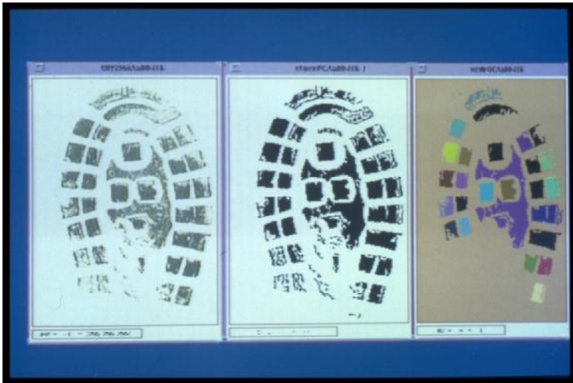
Figure 5-9 : Example of segmenting and labeling a shoe mark
