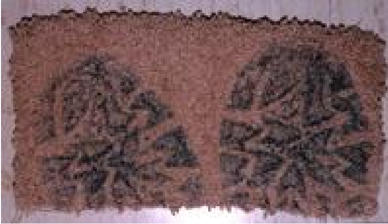
Figure 5-1 : Latent shoe mark on carpet that is treated with Leuco Crystal Violet
