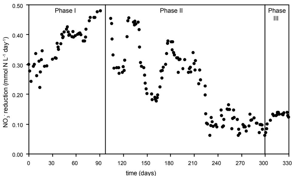
**Figure 1:** NO<sub>3</sub><sup>-</sup> reduction (in mmol N L<sup>-1</sup> day<sup>-1</sup>) in a denitrifying bioreactor at pH 4 over time. During phase I no electron donors were supplied, during phase II naturally available electron donors were supplied, at the start of phase III, the pH was increased to 6.
