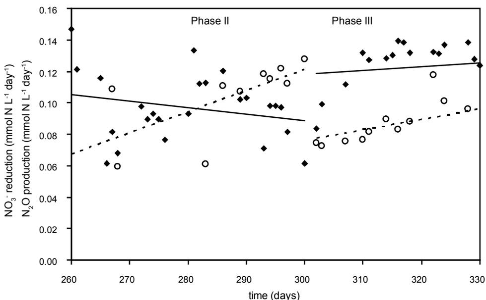
**Figure 2:**  $\text{NO}_3^-$  reduction and  $\text{N}_2\text{O}$  production in the denitrifying bioreactor before and after a switch in pH.  $\text{NO}_3^-$  reduction (black diamonds, solid trendlines, in  $\text{mmol L}^{-1} \text{ day}^{-1}$ ) and  $\text{N}_2\text{O}$  production (open circles, dotted trendlines, in  $\text{mmol N L}^{-1} \text{ day}^{-1}$ ) over time. The pH of the reactor was increased from 4.0 to 6.0 on day 301.
