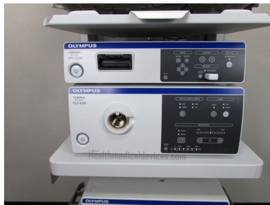
Figure 3. Olympus UM OTV-S190 video processor (top) and Olympus UM CLV-S190 light source (bottom).
