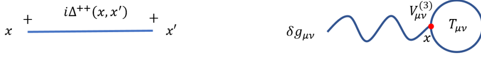
Figure 5: On the left one sees the ++ propagator, which has been calculated in the previous subsection far. On the right the expression for the energy momentum tensor is shown. The wiggly line corresponds to the metric and the solid lines correspond to the scalar field. The red dot denotes the three point vertex V_{\mu\nu}^{(3)} . One obtains a loop in the diagram because one takes the limit x \rightarrow x' . In this thesis one only calculates the energy momentum tensor up to the tadpole order.
