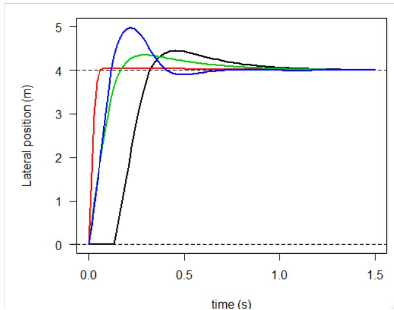
**Figure 6.** Individual steering profiles predicted by the model. The goal of the model is to steer four meters to the left, beginning at time 0. Black: high  $t_0$ ; green: high  $k_f$ , Red: high  $k_n$ , Blue: High  $k_I$ .
