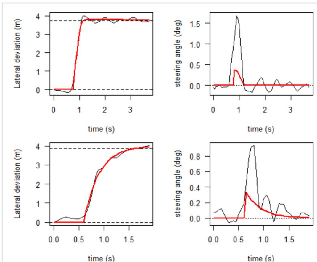
**Figure 7.** Two example participants with different steering profiles are fit by the model. Left: Observed (black) and predicted lateral deviation from the initial road location. Dashed lines indicate the initial road location and the final road location. Right: Observed (black) and predicted (red) steering angle. Dotted line indicates that steering wheel is in the upright position.
