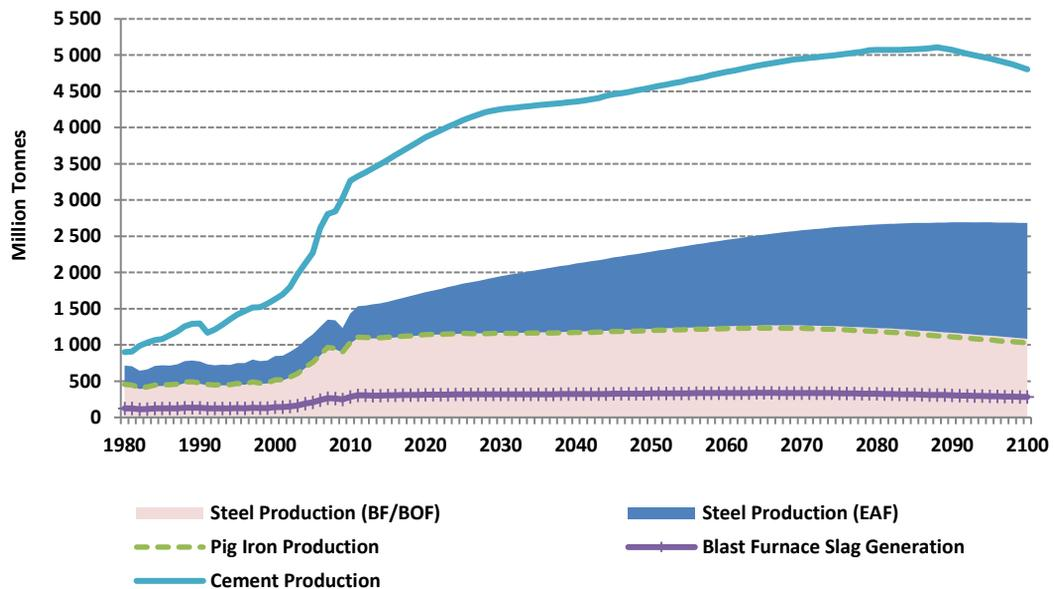
**Figure 3:** Projections of global cement demand, steel production, pig iron production and blast furnace slag generation (author own calculations)<sup>23,24</sup>
