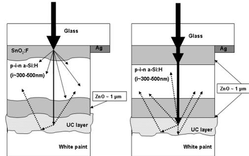
**Figure 2:** Schematic overview of the two solar cell designs used in these experiments. In flat solar cells the incoming light is not scattered and much higher light density reaches the upconverter layer by placing the interference maximum for the relevant wavelength at the upconverter. The increase in light intensity should lead to a nearly quadratic increase in upconverter response.
