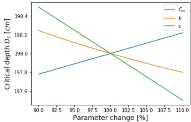
Figure 2: Sensitivity analysis for parameters  $C_{ss}$ ,  $k$  and  $c$  for the critical depth  $D_c$ . A higher suspended sediment concentration causes the critical depth to increase, whereas a higher vegetation growth and plant sediment capture leads to a lower critical depth.
