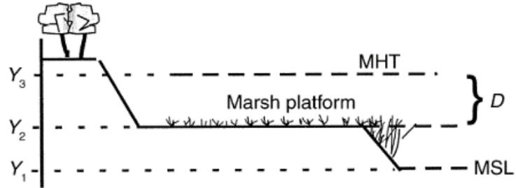
Figure 1: The depiction of mean high tide ( $Y_3$ ), the saltmarsh height ( $Y_2$ ) and the mean sea level ( $Y_1$ ) relative to each other (Morris et al., 2002). The depth  $D$  is given by  $D = Y_3 - Y_2$ .
