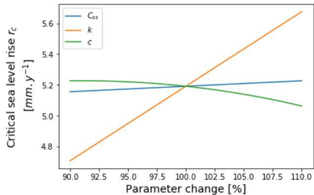
Figure 3: Sensitivity analysis for parameters  $C_{ss}$ ,  $k$  and  $c$  for the critical rate of sea level rise  $r_c$ . A higher suspended sediment concentration and a higher plant sediment capture leads to a higher critical sea level rise, whereas an increase in vegetation growth leads to a lower critical sea level rise.
