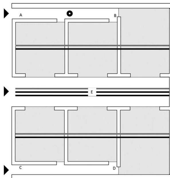
**FIGURE 1** A map of 1 of the 4 identical stable units. The black circle indicates the standard location for sampling. The letters A-E indicate the locations where the variable samples were taken. The arrow heads indicate doors, with the middle door being an important inlet for fresh air. The gray lines indicate the corona wires, and the black lines indicate the iron wires required to create sufficient earthed surface
