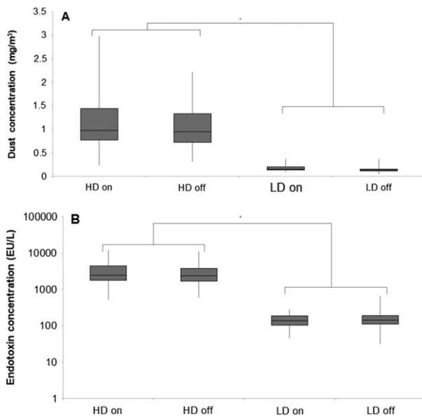
**FIGURE 3** Boxplots of dust concentrations (A) and endotoxin concentrations (B) in horse stables with different types of bedding and feed and with and without ionization; “on” and “off” indicating whether ionization was operating or not; HD, high dust unit with straw bedding and dry hay feeding; LD, units with shavings bedding and haylage feeding; \* = significant different to HD units
