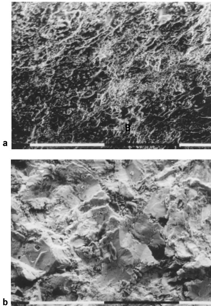
“rounded/smooth”-like surface as a result of the vacuum plasma-spraying, while on the surface of the Ti implants clearly the sharp edges, as a result of the grit blasting procedure, are visible.
