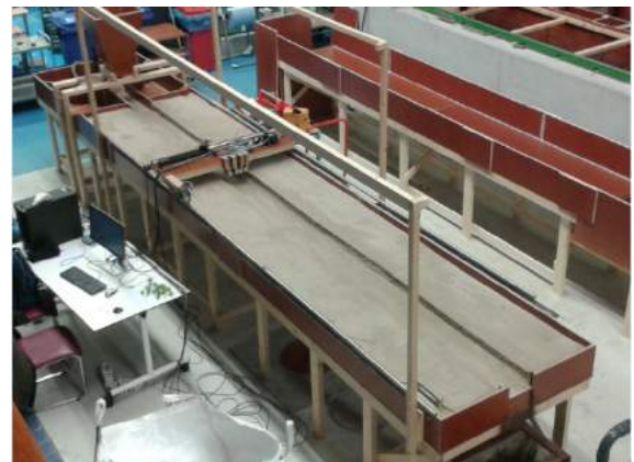
Figure 13. Sand-bed flume, with sediment feeder in the upstream and laser recorders.
