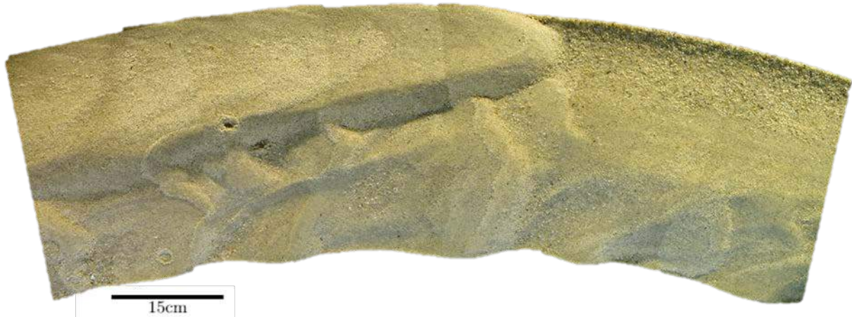
Figure 25 Top view of a section of the bed in the annular flume. Flow was from left to right. In the outer bend, there is a dune top, followed by a coarse trough. In the inner bend, there are ripples that collapse downstream of the dune's brinkpoint.
