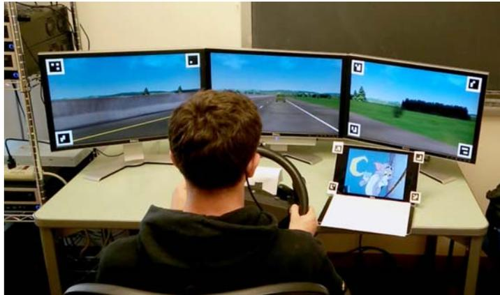
**Figure 2. Overview of the DriveSafety driving simulator and the distraction video with the markers which the eye tracker can use as landmarks.**
