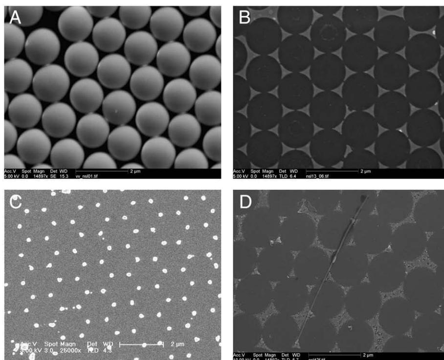
**Fig. 1.** (A) Silica spheres of  $(1400 \pm 20)$  nm used as a monolayer deposition mask. (B) An array of nickel prisms residues after sonication. (C) Annealing deforms the prisms into round dots. (D) A secondary electron picture of isolated carbon nanofiber formation. All pictures are made with SEM.
