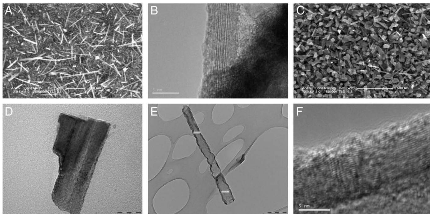
**Fig. 2.** (A) Nanostructures with  $(10 \pm 4)$  nm thickness and mostly shorter than 500 nm. (B) A HRTEM picture of a 6.5 nm wide nanostructure. (C) Flake-like structures. (D) A TEM picture of a flake. The scale bar is 20 nm. (E) A TEM image of a  $\sim 100$  nm thick and 1.2  $\mu\text{m}$  long MWCNT. The scale bar is 200 nm. (F) HRTEM picture of one of the walls of the MWCNT in Figure (E) showing graphene layers. All pictures are made with SEM or TEM.
