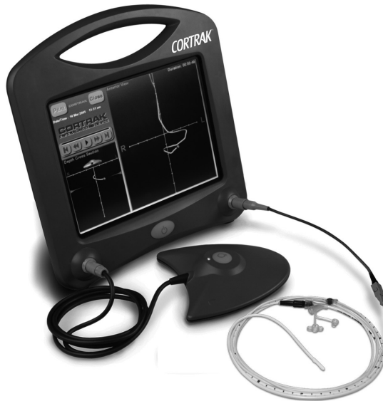
Figure 1 The Cortrak® Enteral Access System (electromagnetic transmitting stylet, receiver unit and enteral feeding tube). The tip of the tube is displayed on the monitor as a dot and the path of the tube is reflected by a yellow line. Image reproduced with permission of CORPAK MedSystems
