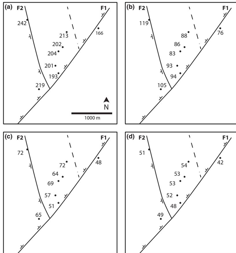
Fig. 6. Thickness maps for the studied stratigraphic interval. (A) complete interval, (B) Unit 1, (C) Unit 2 and (D) Unit 3.
