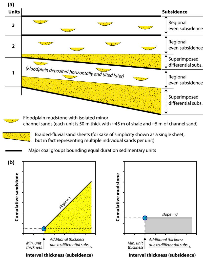
**Fig. 8.** Diagram showing (A) the overall distribution of braided-fluvial sands and coal-bearing floodplain deposits in Units 1, 2 and 3; and (B) cross-plot trends for cumulative-sandstone and cumulative-mudstone thickness.
