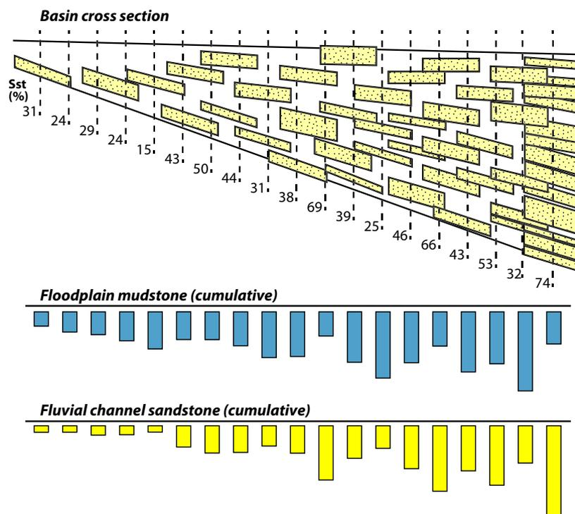
**Fig. 1.** Half-graben cross-section showing the distribution of fluvial channels (redrawn after Bridge & Mackey, 1993). Sandstone percentage, cumulative-sandstone and cumulative-mudstone thickness are indicated.
