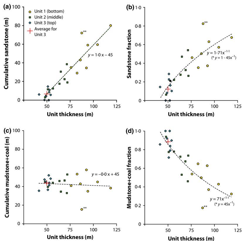
**Fig. 7.** Cross-plots of lithological thickness data versus cycle thickness. (A) cumulative-sandstone thickness, (B) sandstone fraction, (C) cumulative-mudstone/coal thickness and (D) mudstone/coal fraction. \*Regression equation with outlier\*\* excluded.
