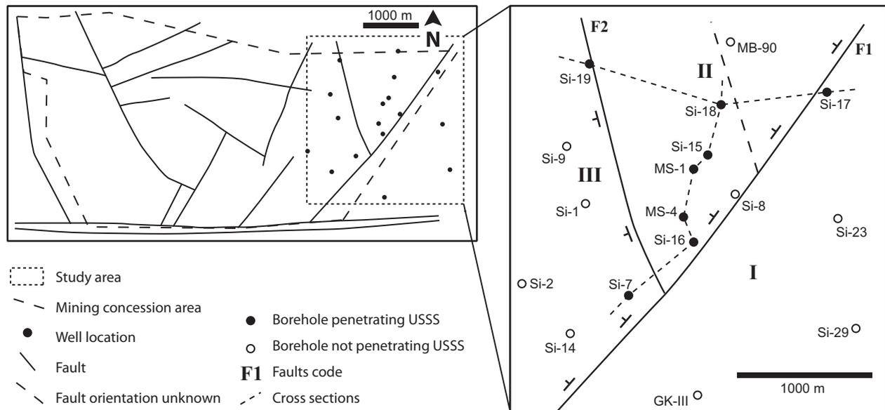
**Fig. 4.** Map of the Silesia mining concession showing major faults and borehole locations for the study area. The study area covers 3 fault blocks (numbered I to III) with densely spaced boreholes. Wells not incorporated in the cross-sections do not penetrate the studied interval or only partly and were therefore not included in the quantitative analysis (open circles).
