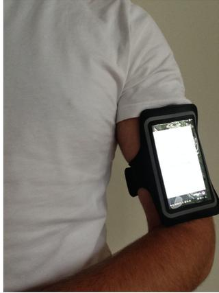
Figure 2: The smartphone worn on the left upper-arm in a running armband.
