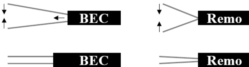
Figure 5: Comparison of the working mechanisms of the Remorgida (Remo) and Bipolar electrocoagulation forceps (BEC).
