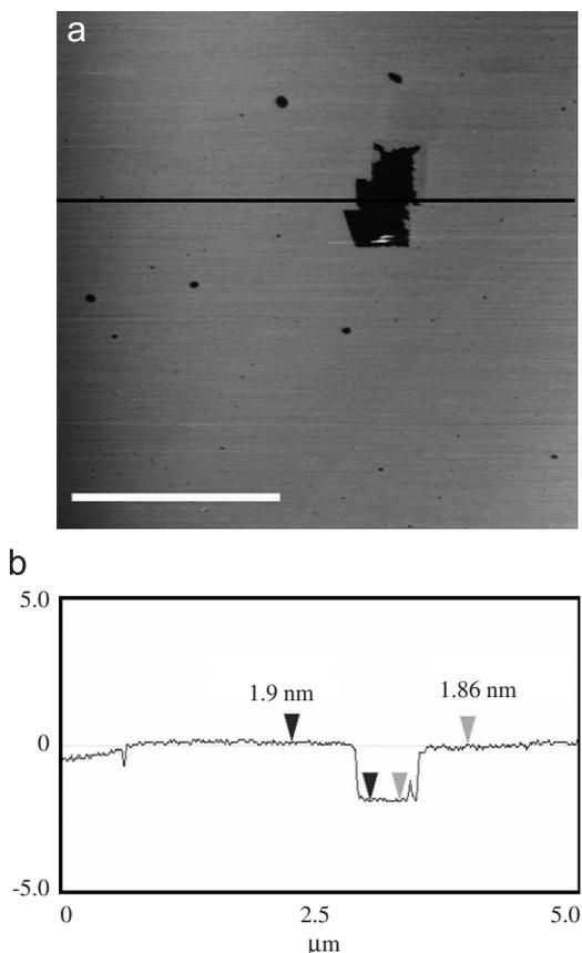
Fig. 6. (a) AFM height image of SSS–AAA (1:1) monolayer transferred immediately after forced compression to  $\pi = 20$  mN/m and the corresponding cross section in (b). The black square is a hole in the monolayer produced by scanning at a high AFM force ( $F \sim 30$  nN). The monolayer is scanned at AFM force  $F \sim 1$  nN. The scale bar is 2  $\mu\text{m}$  and the vertical scale is 10 nm. Height differences are given by the numbers at the markers.
