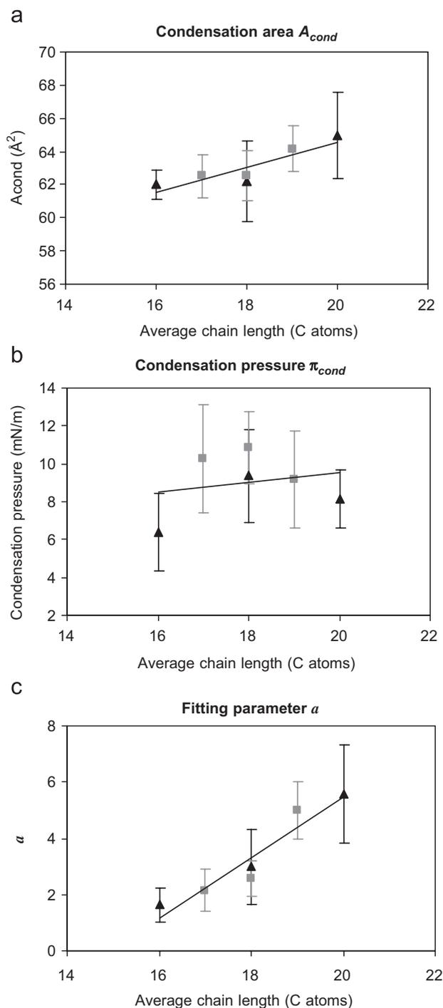
Fig. 2.  $A_{\text{cond}}$  (a),  $\pi_{\text{cond}}$  (b) and fitting parameter  $a$  (c) for triglycerides ( $\blacktriangle$ ) and their mixtures ( $\blacksquare$ ). X-axis presents the number of the carbon atoms in the triglyceride chains: PPP (16), SSS (18) and AAA (20). For the mixtures it was calculated as follow: 17 = PPP–SSS (1:1), 18 = PPP–AAA (1:1) and 19 = SSS–AAA (1:1).
