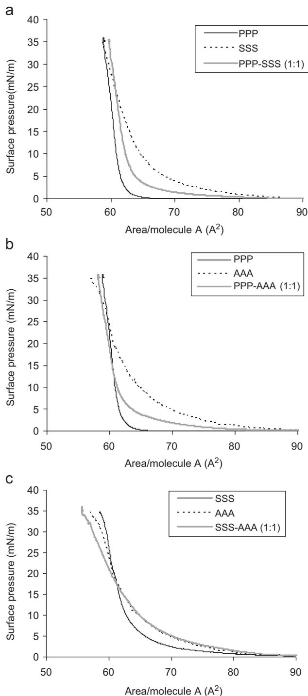
Fig. 1. Surface pressure vs area isotherms of tripalmitin (PPP), tristearin (SSS) and triarachidin (AAA) and their mixtures at air–water interface, at 20 °C, obtained by forced compression at a rate of 1 cm/min.
