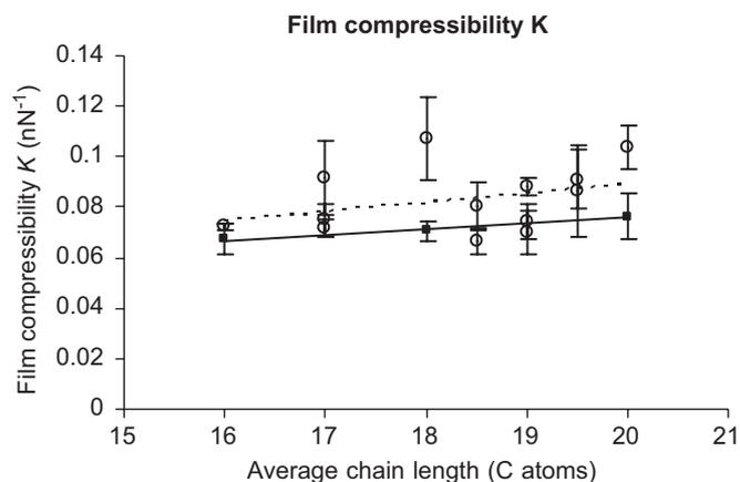
Fig. 13. Film compressibility  $\tilde{K}$  as a function of the chain length for the pure components (■) and their mixtures (○).
