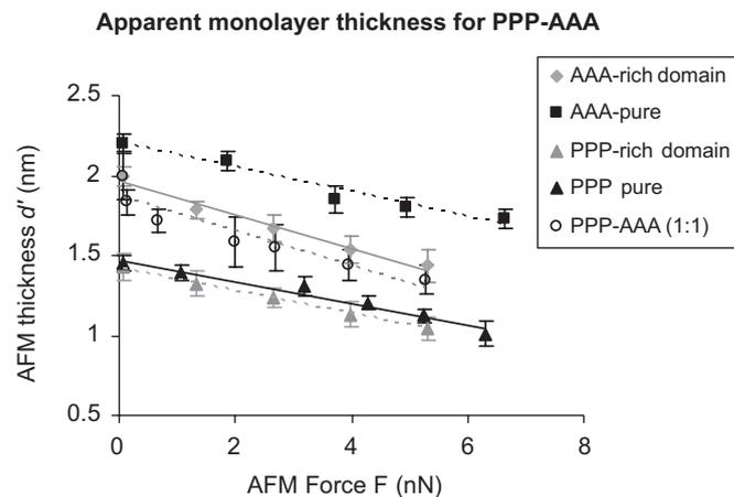
Fig. 10. Measured layer thickness  $d'$  for PPP, AAA from the monolayers of the pure components and in the mixture PPP–AAA (1:1) as a function of applied AFM force  $F$  at surface pressure  $\pi = 20$  mN/m.
