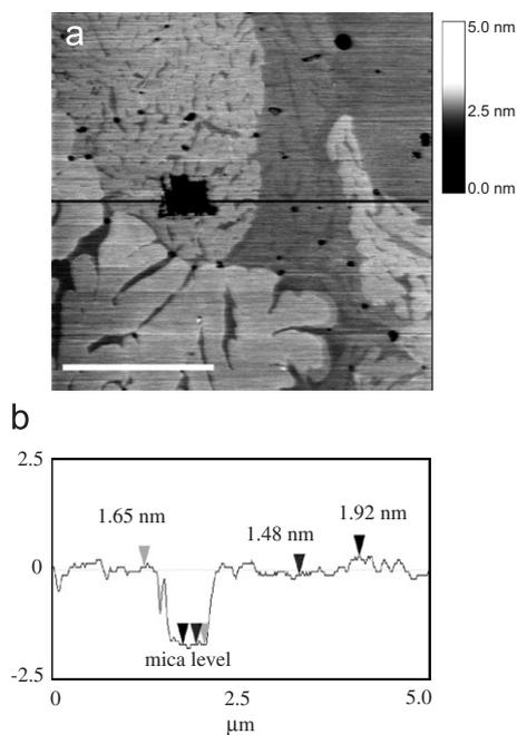
Fig. 11. (a) AFM height image of PPP–AAA (1:1) monolayer transferred immediately after forced compression to  $\pi = 20$  mN/m. The corresponding cross section in (b) presents three different domains in the mixture. The black square is a hole in the monolayer produced by scanning at a high AFM force ( $F \sim 30$  nN). The monolayer is scanned at AFM force  $F \sim 1$  nN. The scale bar is  $2 \mu\text{m}$ . Height differences are given by the numbers at the markers.
