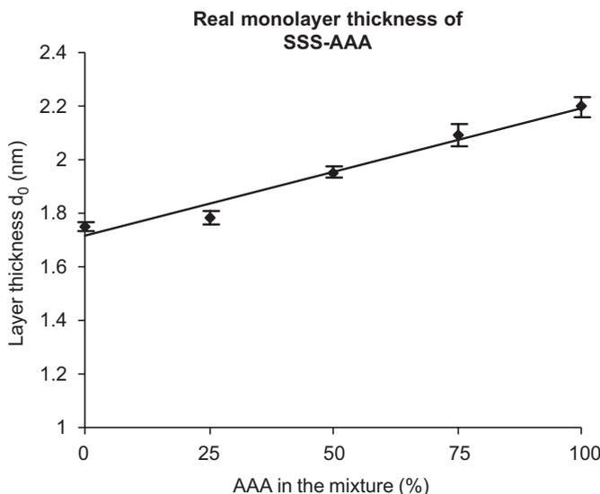
Fig. 8. Real monolayer thickness  $d_0$  for SSS–AAA at surface pressure  $\pi = 20$  mN/m as a function of the mole fraction of AAA in the mixture. The values are found by extrapolation of the apparent monolayer thickness  $d'$  to AFM force  $F = 0$  nN.
