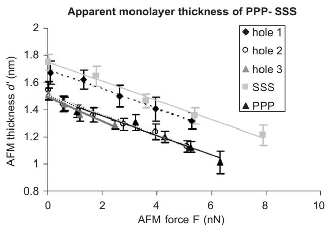
Fig. 4. Measured layer thickness  $d'$  for PPP, SSS and PPP–SSS (1:1) as a function of applied AFM force  $F$  at surface pressure  $\pi = 20$  mN/m.
