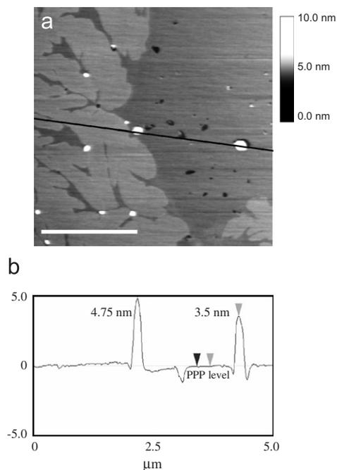
Fig. 12. AFM height image of PPP–AAA (1:1) monolayer transferred immediately after forced compression to  $\pi = 20$  mN/m (a) and the corresponding cross section in (b). The image presents crystals on top of the monolayer. Their height is measured from the PPP level. The scale bar is  $2 \mu\text{m}$ . Height differences are given by the numbers at the markers.
