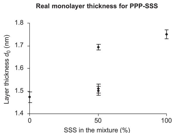
Fig. 5. Real monolayer thickness  $d_0$  for PPP, SSS and PPP–SSS (1:1) for three different holes at surface pressure  $\pi = 20$  mN/m. The  $d_0$  values are found by extrapolation of the apparent monolayer thickness  $d'$  in Fig. 4 to AFM force  $F = 0$  nN.
