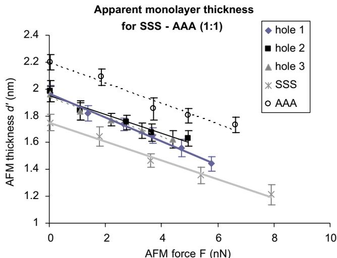
Fig. 7. Measured layer thickness  $d'$  for SSS, AAA and SSS–AAA (1:1) as a function of applied AFM force  $F$  at surface pressure  $\pi = 20$  mN/m.
