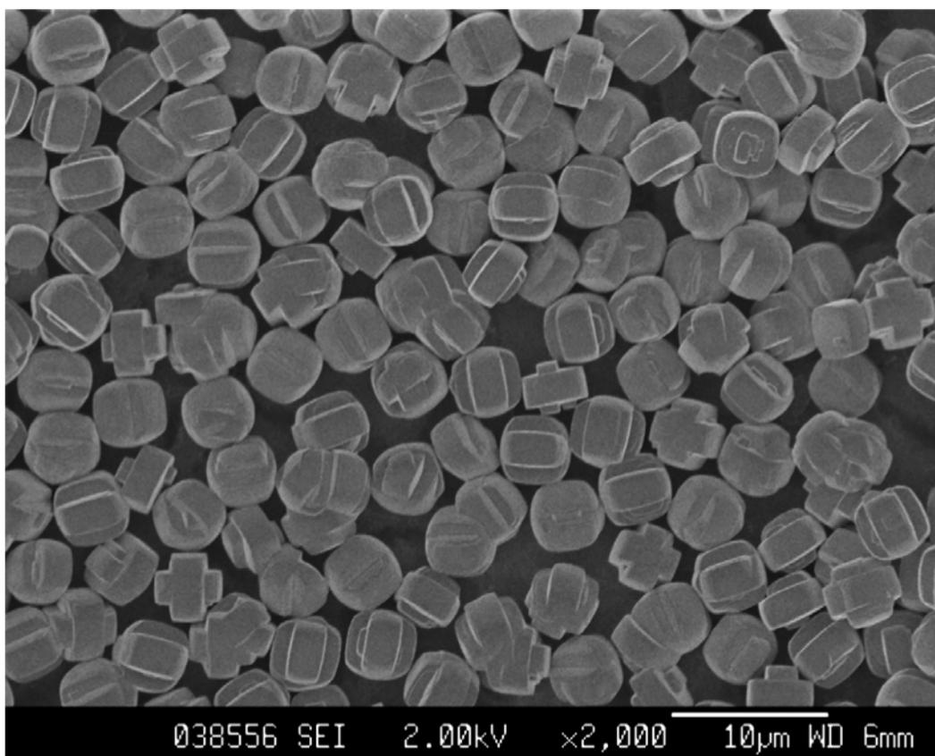
**Figure 1.** SEM image of our silicalite sample.
