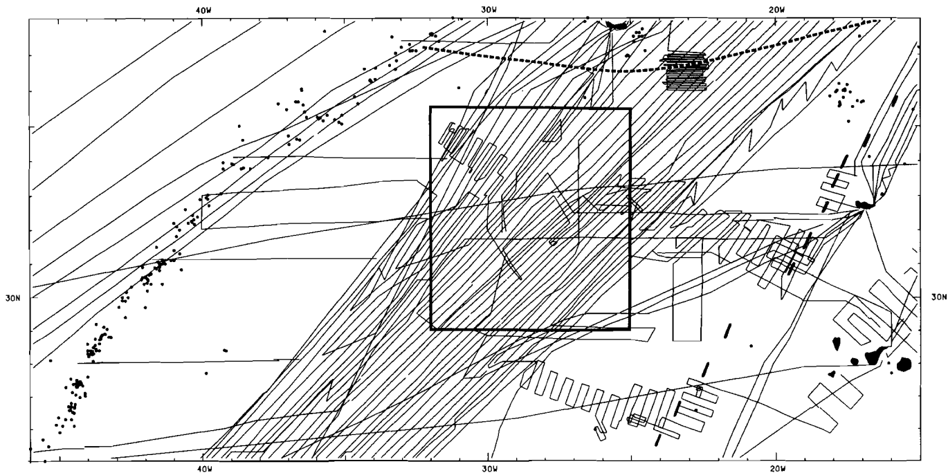
Figure 1: Tracklines with seismic data. The heavy dashes give the East Azores fracture zone, which forms the northern boundary of the study area. The discontinuous heavy line indicate the Mesozoic magnetic anomaly MO (eastern boundary). The Mid-Atlantic ridge is indicated by the earthquake epicenters (western boundary). The central square indicates the seamount area, studied in chapter 2.
