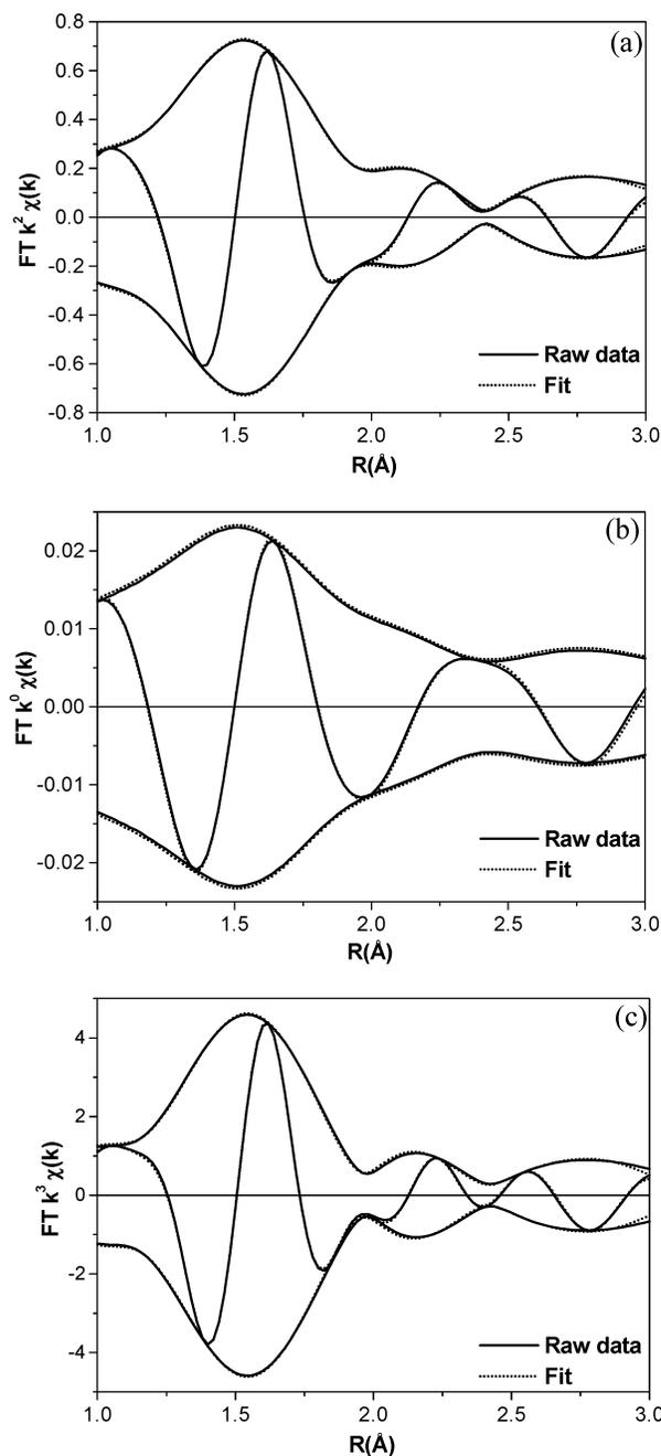
**Figure 4.** Fourier transforms of raw data and  $R$ -space fit ( $4 < k < 12 \text{ \AA}^{-1}$  and  $1 < R < 3 \text{ \AA}$ ) of CZ-31-0.58 treated in  $O_2$  at 623 K and measured at LN (a)  $k^2$ -, (b)  $k^0$ -, and (c)  $k^3$ -weighted.
