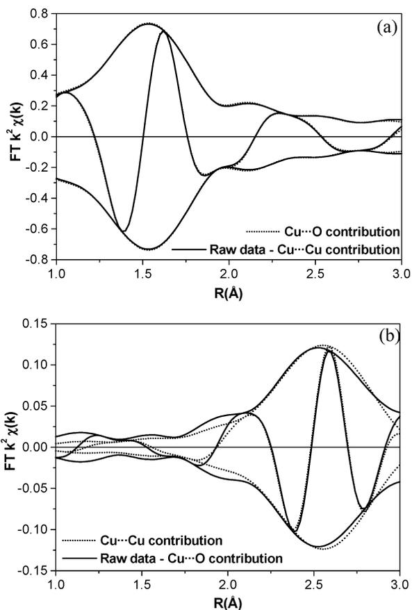
**Figure 5.** Fourier transforms of fitted single shell contributions (dotted line) and difference files (solid line) of  $R$ -space fit ( $k^2$ ,  $4 < k < 12 \text{ \AA}^{-1}$ , and  $1 < R < 3 \text{ \AA}$ ) of CZ-31-0.58 treated in  $\text{O}_2$  at 623 K and measured at LN (a) Cu...O and (b) Cu...Cu.
