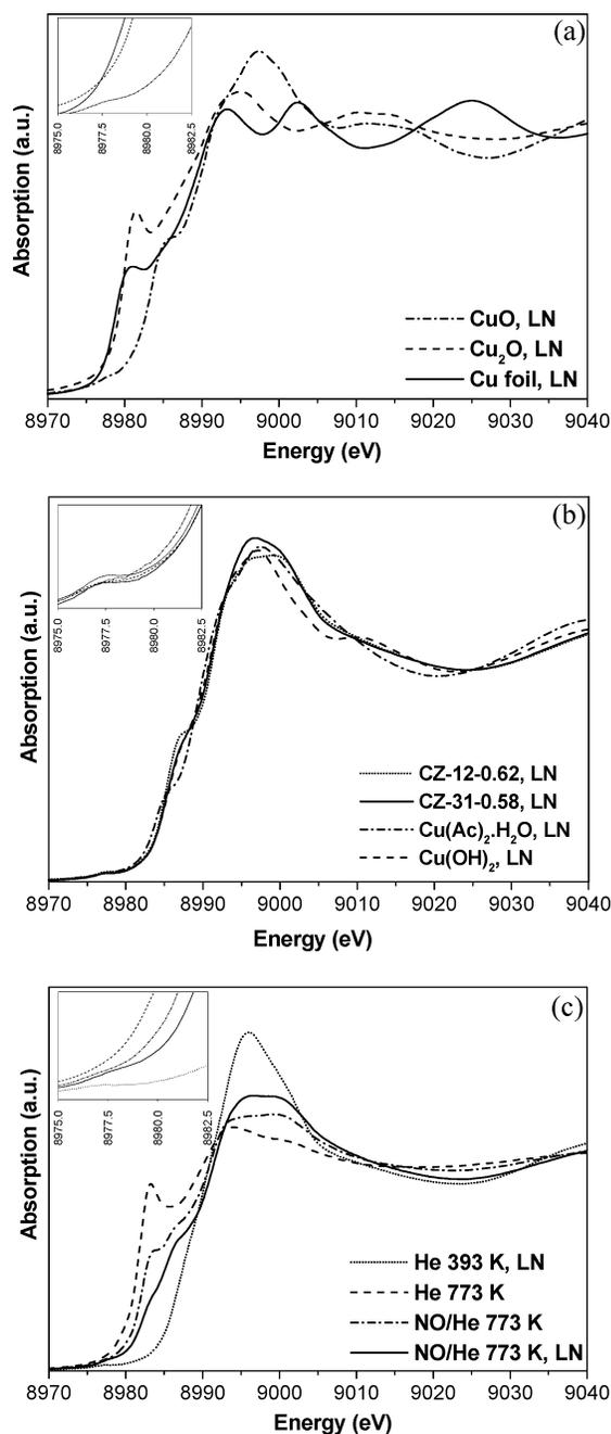
**Figure 2.** XANES spectra of (a) CuO, Cu<sub>2</sub>O, and Cu foil at LN; (b) CZ-12-0.62 and CZ-31-0.58 treated in O<sub>2</sub> at 623 K and of copper(II) acetate monohydrate and Cu(OH)<sub>2</sub> measured at LN; (c) CZ-12-0.62 (i) treated in He at 393 K and measured at LN, (ii) treated in He at 773 K and measured at 773 K, (iii) treated in NO/He at 773 K and measured at 773 K, and (iv) treated in NO/He at 773 K and measured at LN.
