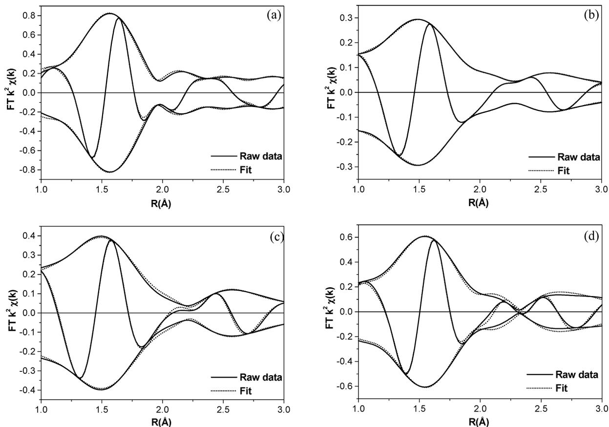
**Figure 7.**  $k^2$ -weighted Fourier transforms of raw data and  $R$ -space fit ( $4 < k < 12 \text{ \AA}^{-1}$  and  $1 < R < 3 \text{ \AA}$ ) of CZ-12-0.62 after (a) treatment at 393 K in He and measured at LN, (b) treatment at 773 K in He and measured at 773 K, (c) treatment at 773 K in NO/He and measured at 773 K, and (d) treatment at 773 K in NO/He and measured at LN.
