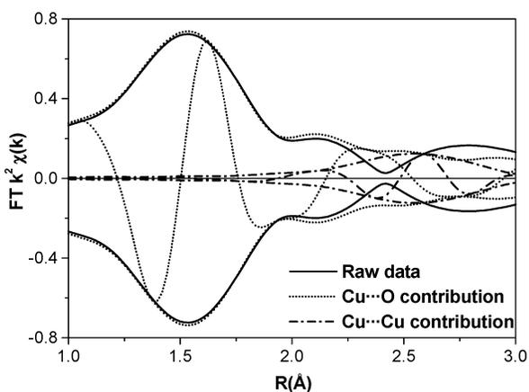
**Figure 6.** Fourier transforms of raw data and fitted single shell contributions of Cu...O and Cu...Cu of  $R$ -space fit ( $k^2$ ,  $4 < k < 12 \text{ \AA}^{-1}$ , and  $1 < R < 3 \text{ \AA}$ ) of CZ-31-0.58 treated in  $\text{O}_2$  at 623 K and measured at LN.
