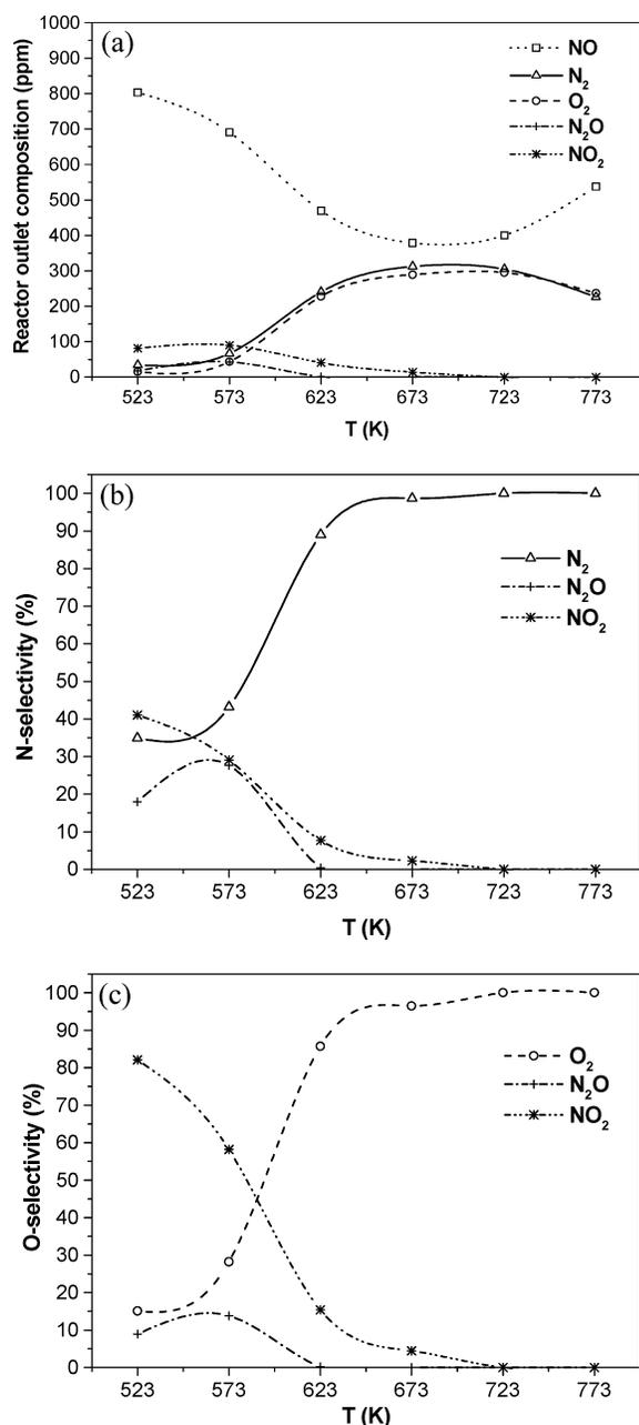
Figure 1. (a) Reactor outlet composition of CZ-12–0.62 contacted with 1000 ppm NO in He at 900 h<sup>-1</sup>; (b) the corresponding N-selectivity and (c) O-selectivity (all as a function of temperature).
