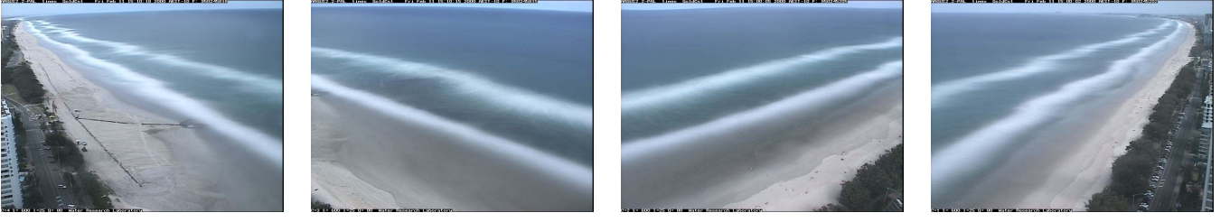
(a) Time-exposure Argus images of all cameras. The high-intensity bands in each image are due to persistent wave breaking on the inner and outer bar.
